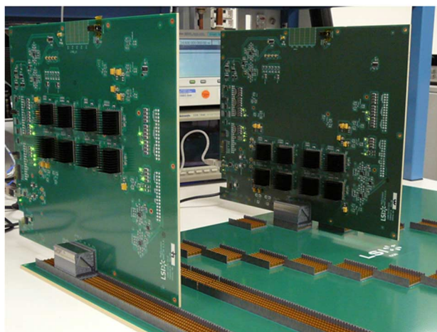
Fig. 24. 100 G Ethernet system implementation.
