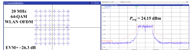
Fig. 25. Measured output spectrum and constellation of 20-MHz 64-QAM WLAN OFDM signal at 2.4 GHz.
