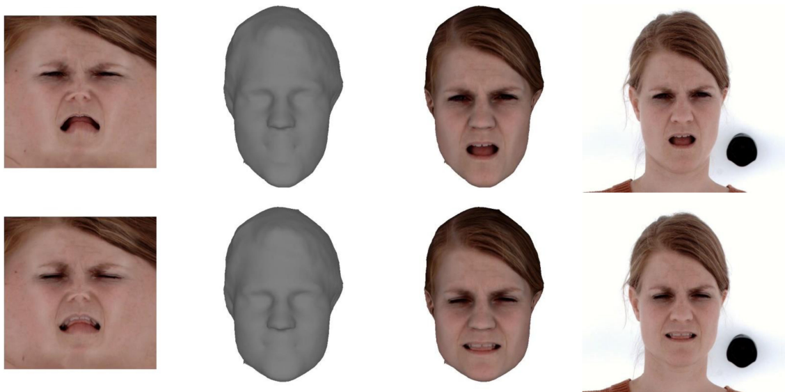
FIGURE 1. Results of the facial performance capture process. Each row shows a different facial expression. From left to right, we show the dynamic face texture, the underlying face geometry, the rendered face model, and the original video frame.
