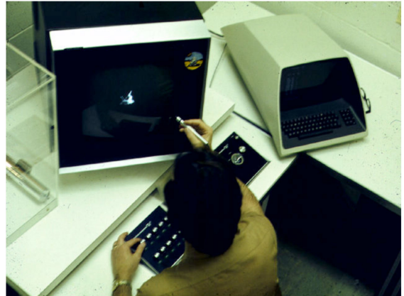
FIGURE 4. Csuri interacting with a light pen at the VG3D display, showing buttons, dials, and joystick. To the left is the sonic pen device, and to the right is the VT100 (photo courtesy of CGRG).
