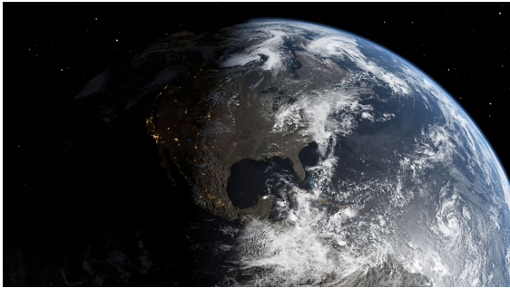
FIGURE 1. Photo-realistic visualization of a global ICON atmosphere simulation at 2.5 km resolution. Clouds are a 2-D composition of vertically integrated liquid cloud water and ice, and rendered using a physically based rendering (PBR) approach.
