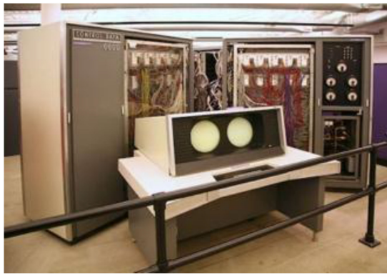
Figure 4. CDC 6600 Mainframe showing typical “spaghetti wiring” (Used under CC by 2.0 license). 10
