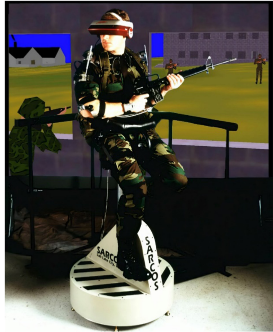
FIGURE 5. The iPort soldier interface. Three virtual Jack models are visible, each dressed in camouflage. On the left is the user's avatar, showing his position and pose in the interface. This avatar was movable anywhere in the scene by user swiveling and pedaling in the iPort. In the upper right, two Jack "combatants" are visible targets for the military simulation. Image courtesy of Mike Zyda.
