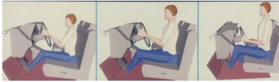
FIGURE 3. Three different size Jack models in an automobile cockpit. The range of size variability from 5th to 95th percentile males is evident. The rightmost image is scaled down slightly to fit the image frame.
