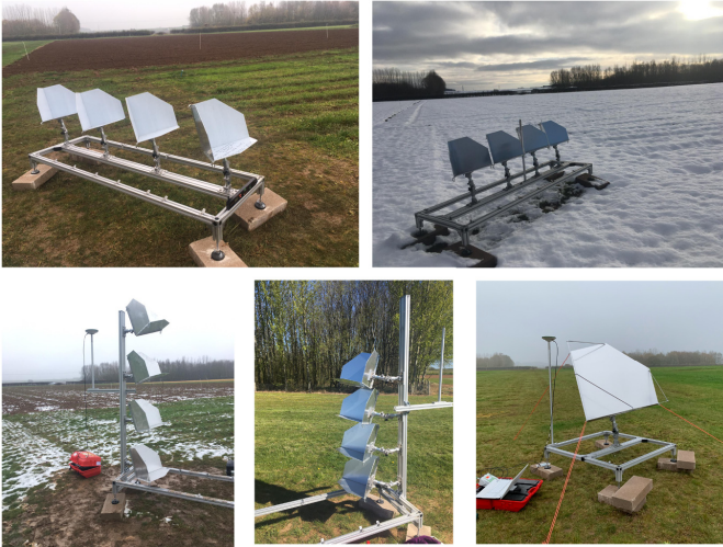
Fig. 10. Photographs of the installation of the various configurations. (Top Left) Alignment in range horizontal. (Top Right) Alignment in azimuth horizontal. (Bottom Left) Alignment in azimuth vertical. (Bottom Middle) Same vertical alignment with shadowing (where the vertical separation is too small to have a clear view of the satellite for the lower three reflectors). (Bottom Right) Large reflector intended as a reference reflector in the field.
