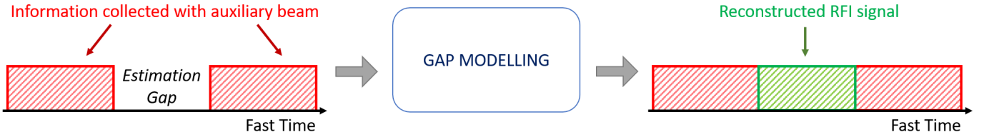
Fig. 9. Information collected with the auxiliary beam (red) is used to model the signal inside the estimation gap.
