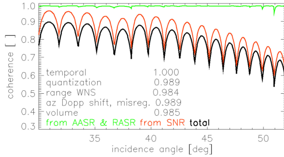
Fig. 21. Summary of all coherence contributions. The total coherence is the lowest curve in black color.
