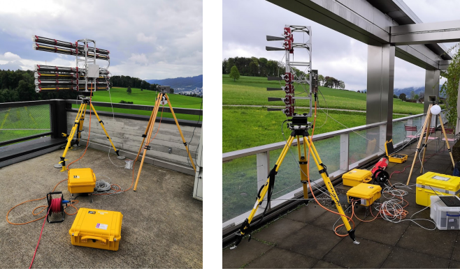
Fig. 3. Bistatic KAPRI device configuration (left: primary device (P) equipped with narrow-beam slotted-waveguide antennas and right: secondary receiver device (S) equipped with horn antennas). Reference link horn antennas are placed on tripods on the right side of the two images, together with long-range Wi-Fi antennas for remote device control.
