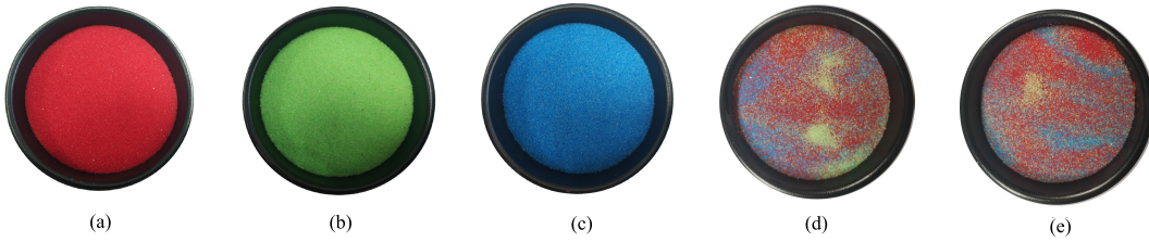
Fig. 8. Laboratory-created data for unmixing performance evaluation (RGB images). (a)–(c) Pure quartz sand with a diameter of 0.3 mm of three colors. They serve as pure materials for providing endmembers. (d) and (e) Mixtures of sand with spatial patterns. Square regions of 60-by-60 pixels in the center of each subfigures are clipped out and used in experiments.
