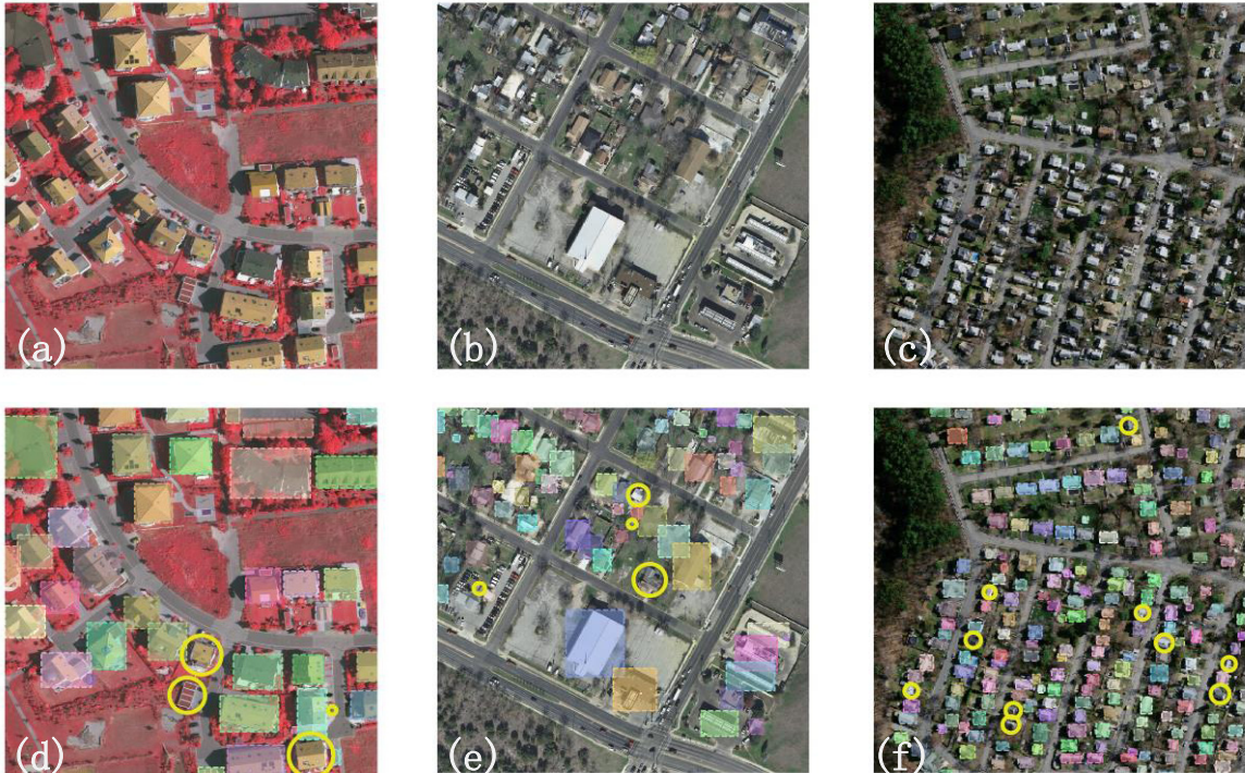
Fig. 9. Results of object detection using the Mask R-CNN. The first row shows three images from the three datasets, respectively, i.e., (a) image of ISPRS, (b) image of INRIA, and (c) image of Massachusetts building datasets. The images coupled with localized buildings are shown in the second row, i.e., (d) object detection results of the image in (a), (e) object detection results of the image in (b), and (f) object detection results of the image in (c).
