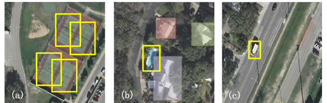
Fig. 10. Result of being incorrectly detected as a building object. (a) Tennis courts. (b) Swimming pool. (c) Large van.
