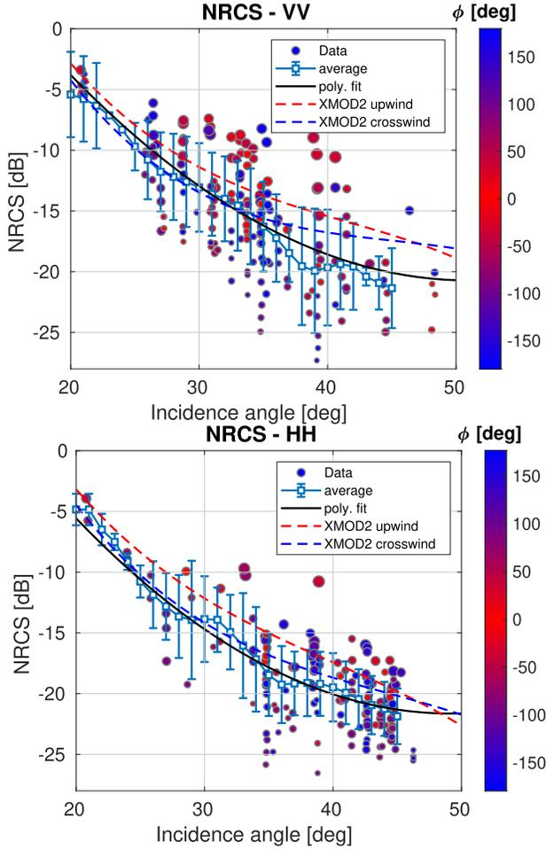
Fig. 9. NRCS dependence on incidence angle for VV (top) and HH (bottom) polarization. Solid lines are the polynomial fit (black) and average (blue) with error bars ( $\pm\sigma_{U_D}$ ). Dashed line is XMOD2 simulated with mean wind speed (5.47 m/s for VV and 5.88 m/s for HH). The size of the data points increases with wind speed from 2 m/s to 15 m/s and the color indicates the relative wind direction (see colorbar).
