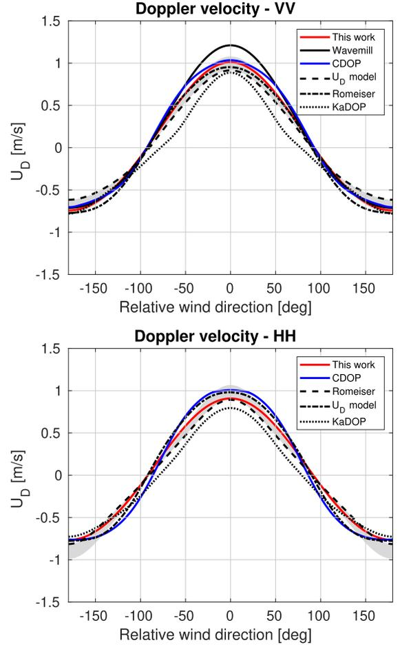
Fig. 14. Comparison against other data sets and models as a function of relative wind direction, for VV (top) and HH (bottom) polarizations. The solid red curve is the  $U_D$  GMF (6) and the dashed black curve is the  $U_D$  model (5). For the other curves see legend. The shaded area is equal to  $(\alpha_1 + \alpha_2)U_{10}$  (see text for details).
