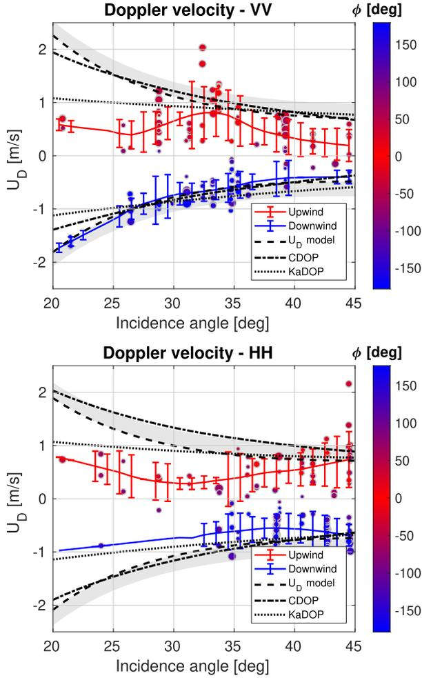
Fig. 11. Estimated  $U_D$  as a function of incidence angle for VV (top) and HH (bottom), all wind speeds and directions included. The size of the data points increases with wind speed from 2 m/s to 15 m/s and the color indicates the relative wind direction (see colorbar). The solid curves represent the average with error bars ( $\pm\sigma_{U_D}$ ). See legend for the other curves.
