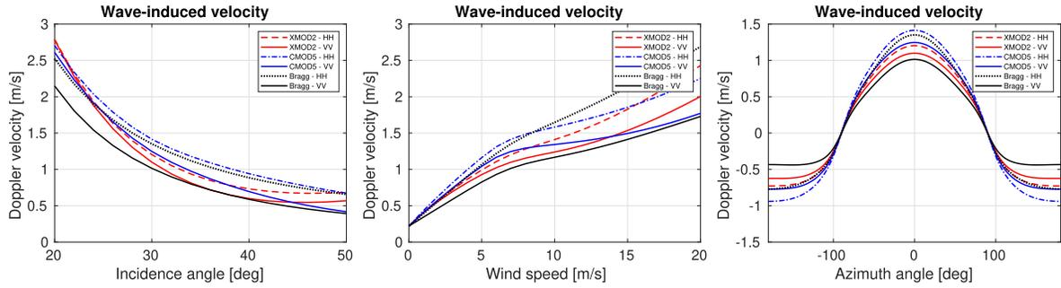
Fig. 4. Comparison of the wave-induced Doppler velocity simulated from tilt MTFs based on different NRCS models (see legend), long wave frequency  $f = 0.15$  Hz, left: as a function of incidence angle ( $U_{10} = 7$  m/s,  $\varphi = 0^\circ$ ), middle: as a function of wind speed ( $\theta = 30^\circ$ ,  $\varphi = 0^\circ$ ), right: as a function of wind direction ( $U_{10} = 7$  m/s,  $\theta = 30^\circ$ ).
