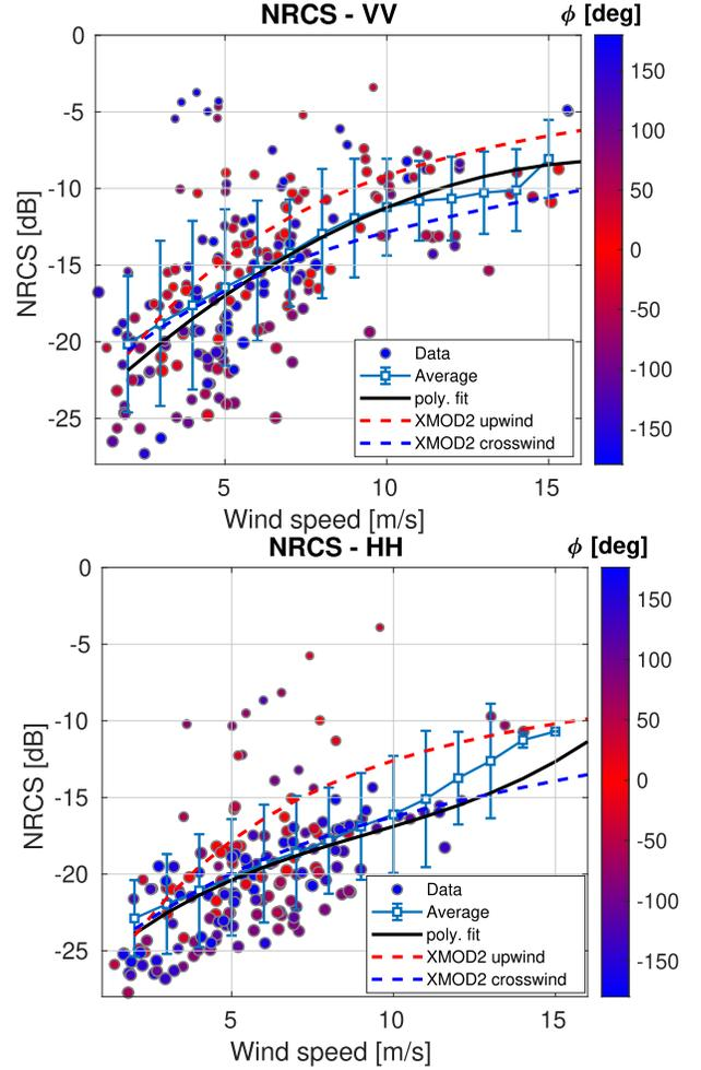
Fig. 10. NRCS dependence on ERA5 wind speed for VV (top) and HH (bottom) polarization. Solid lines are the polynomial fit (black) and average (blue) with error bars ( $\pm\sigma_{U_D}$ ). Dashed line is XMOD2 simulated with mean incidence angle (33.7° for VV and 40° for HH). The size of data points increases with incidence angle from 20° to 50° and the color indicates the relative wind direction (see colorbar).
