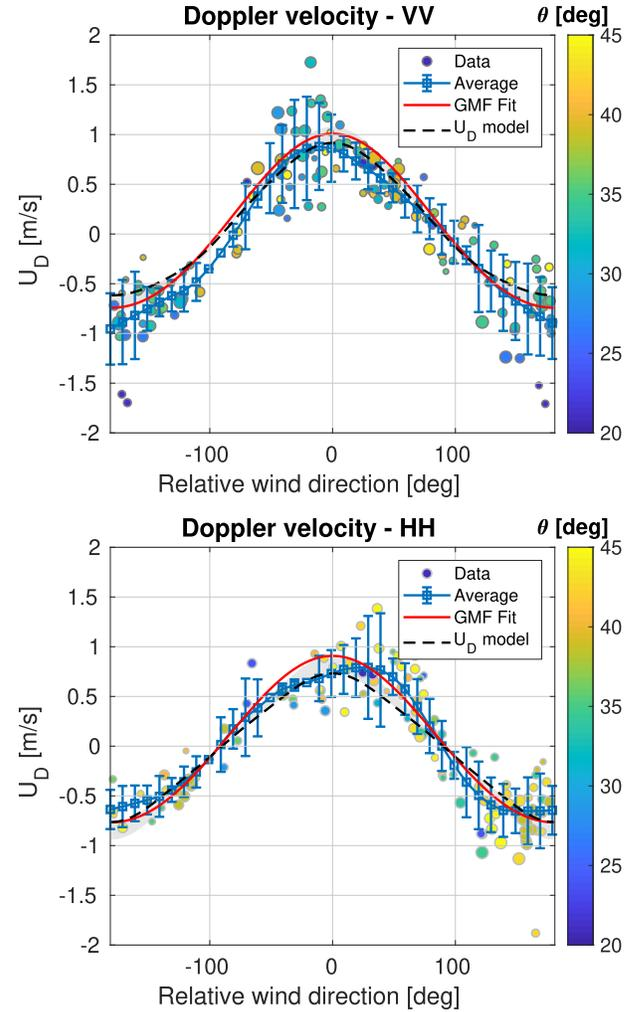
Fig. 13. Estimated  $U_D$  as a function of relative wind direction, for VV (top) and HH (bottom) polarization, all incidence angles and wind speeds included. The size of the data points increases with wind speed from 2 m/s to 15 m/s and the color indicates incidence angle (see colorbar). The blue curve represents the average with error bars ( $\pm\sigma_{U_D}$ ), the red curve is the GMF fit (6) and the dashed curve is the  $U_D$  model (5).
