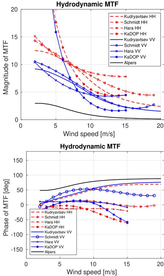
Fig. 2. Hydrodynamic MTF, upper panel: magnitude, lower panel: phase, from different models and experiments (see legend), at X-band,  $\theta = 45^\circ$ ,  $f = \omega/2\pi = 0.15$  Hz, upwave ( $\phi = 0^\circ$ ).
