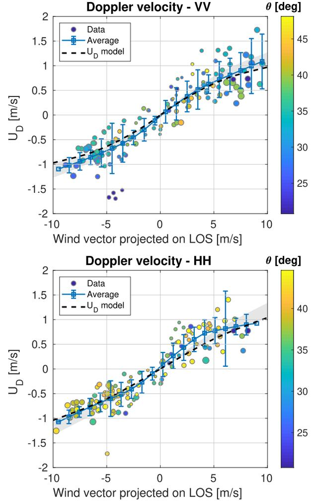
Fig. 12. Estimated  $U_D$  as a function of the radial wind, for VV (top) and HH (bottom) polarization, all incidence angles included. The size of the data points increases with wind speed from 2 m/s to 15 m/s and the color indicates incidence angle (see colorbar). The solid curve represents the average with error bars ( $\pm\sigma_{U_D}$ ) and the dashed curve represents the  $U_D$  model (5).
