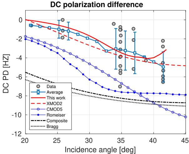
Fig. 17. DC polarization difference ( $PD = |dc_{VV}| - |dc_{HH}|$ ). Measured dc (circles) and average curve with error bars (solid cyan). PD using tilt MTF calculated from, dual-pol NRCS data (solid red), XMOD2 (dashed red), CMOD5 (solid blue with circles), composite surface model (dashed black), pure Bragg model (dotted black), PD from M4S model [15] (solid blue with dots).
