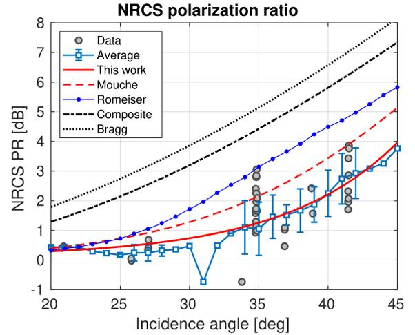
Fig. 16. Polarization ratio ( $PR = \sigma_{VV}^0 / \sigma_{HH}^0$ ). Measured PR (circles) and average curve with error bars (solid cyan), empirical fit to the data (solid red), empirical model from [57] (dashed red), numerical model from [21] (solid blue with dots), composite surface model (dashed black), pure Bragg model (dotted black).
