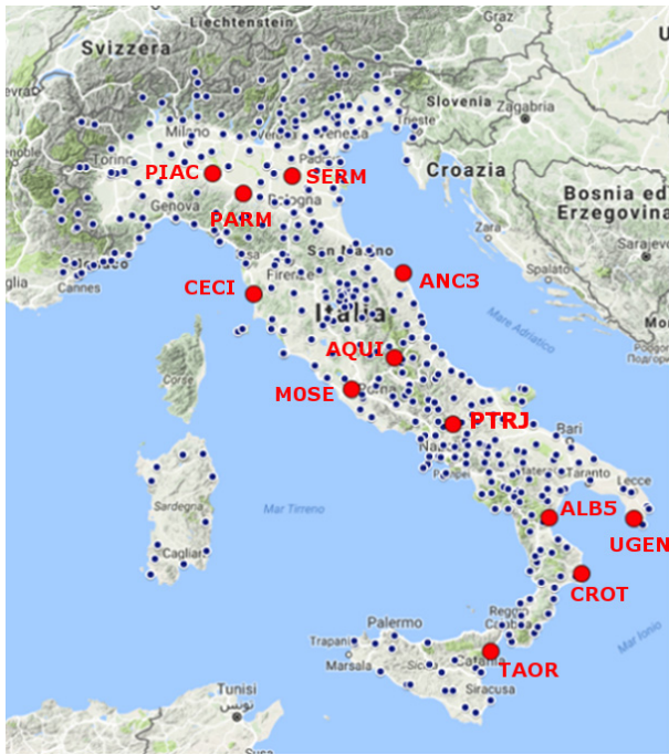
Fig. 14. Google base map of Italian territory with highlighted the locations of the GPS stations (blue and red dots) exploited through the UNR-NGL “Plug and Play GPS” Portal.
