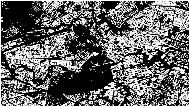
Fig. 7. Automatically generated mask of building regions using OSM + TomoSAR point clouds for the SAR intensity image shown in Fig. 6.
