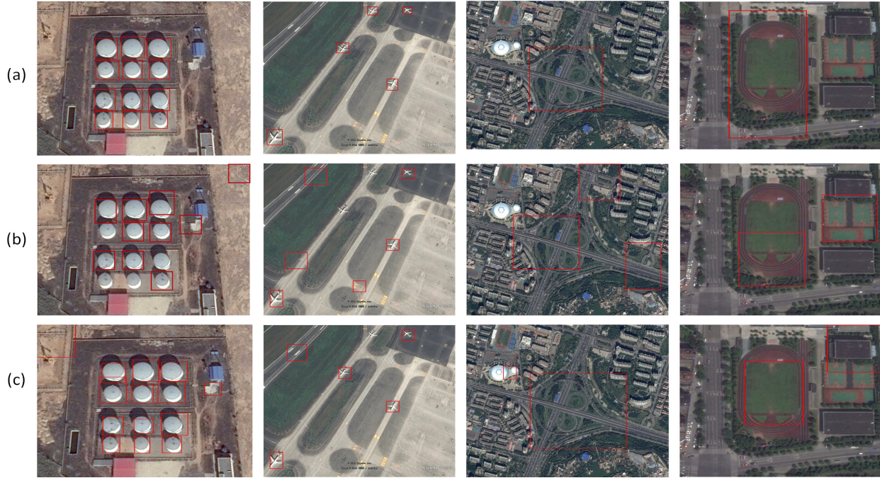
Fig. 5. Comparison of the detection results for the CNN, LBP-HF, and EFT-HOG methods. From left to right, the results are for oil tanks, aircraft, overpasses, and playgrounds. (a) Detection results of the CNN method. (b) Detection results of the LBP-HF method. (c) Detection results of the EFT-HOG method.
