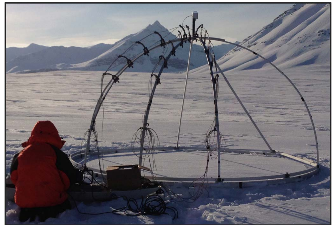
Fig. 2. GRASS with 15 foreoptics mounted on three arms and one foreoptic positioned in the nadir view position. There is an integrating cosine irradiance collector mounted and leveled on the top of the structure. The spectrometer, multiplexer, and laptop are situated in the sled (left), and the all-sky camera is mounted and leveled on a tripod (out of view). Note that no measurement of HDRF was taken at the time this image was captured.
