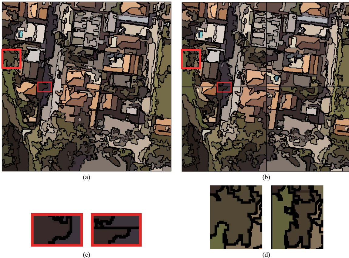
Fig. 1. Impact of image tiling. (a) Represents the output obtained from the reference segmentation of the whole image at once. (b) Represents the output from the tile-based segmentation of the image. The image has been divided into 4 tiles of 250 \times 250 pixels. (c) Shows the presence of an artifact on a tile border due to the fact that segments containing pixels along the tile edges are forced to have their contour along the tile edges. (d) Shows a different segment from the test segmentation compared to the one obtained from the reference segmentation due to the absence of knowledge of segments in other tiles. (a) Segmentation without tiling. (b) Tiled segmentation. (c) Example of an artifact. (d) Different segments.
