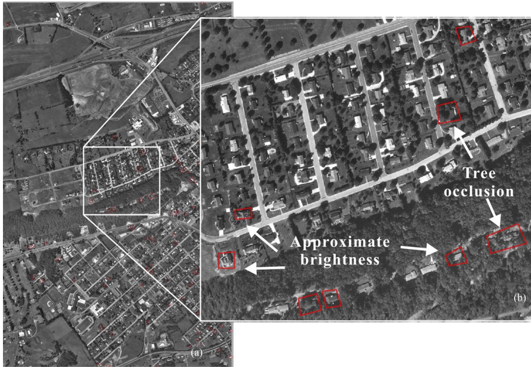
Fig. 25. Tree occlusion impact analysis to the proposed method and the undetected houses.
