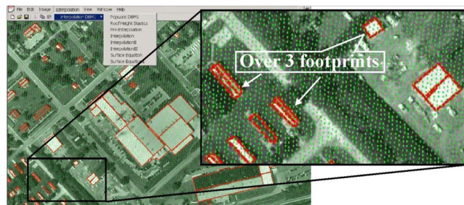
Fig. 21. Coregistration of aerial imagery and LiDAR footprints.
