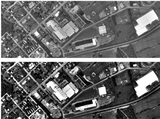
Fig. 14. (a) Original image and (b) enhanced image using a 3 times 3 filtering algorithm.
