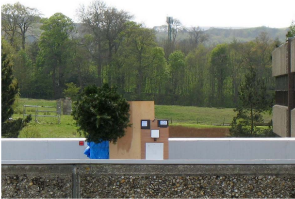
Fig. 2. Photograph showing a small conifer sample used for the experiments described here and several calibration targets, including the Spectralon panel.
