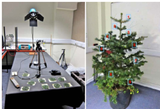
Fig. 7. Passive measurement of the tree sample for validation. On the left are shown the stabilized light source and tripod-mounted spectrometer, with the several needle samples. On the right are shown the tree sample and the marked positions where the nine sets of needle samples were taken from the tree. Four bark samples were also taken.
