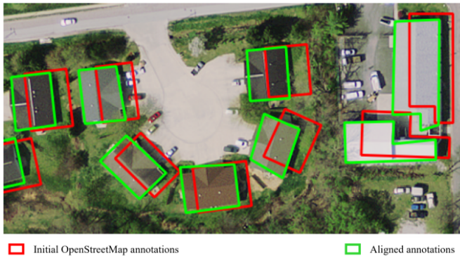
Fig. 11. Aerial imagery with alignment results obtained by the method described in [142].
