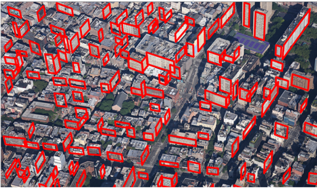
Fig. 3. Off-nadir optical imagery with building facades extracted by the method described in [92].
