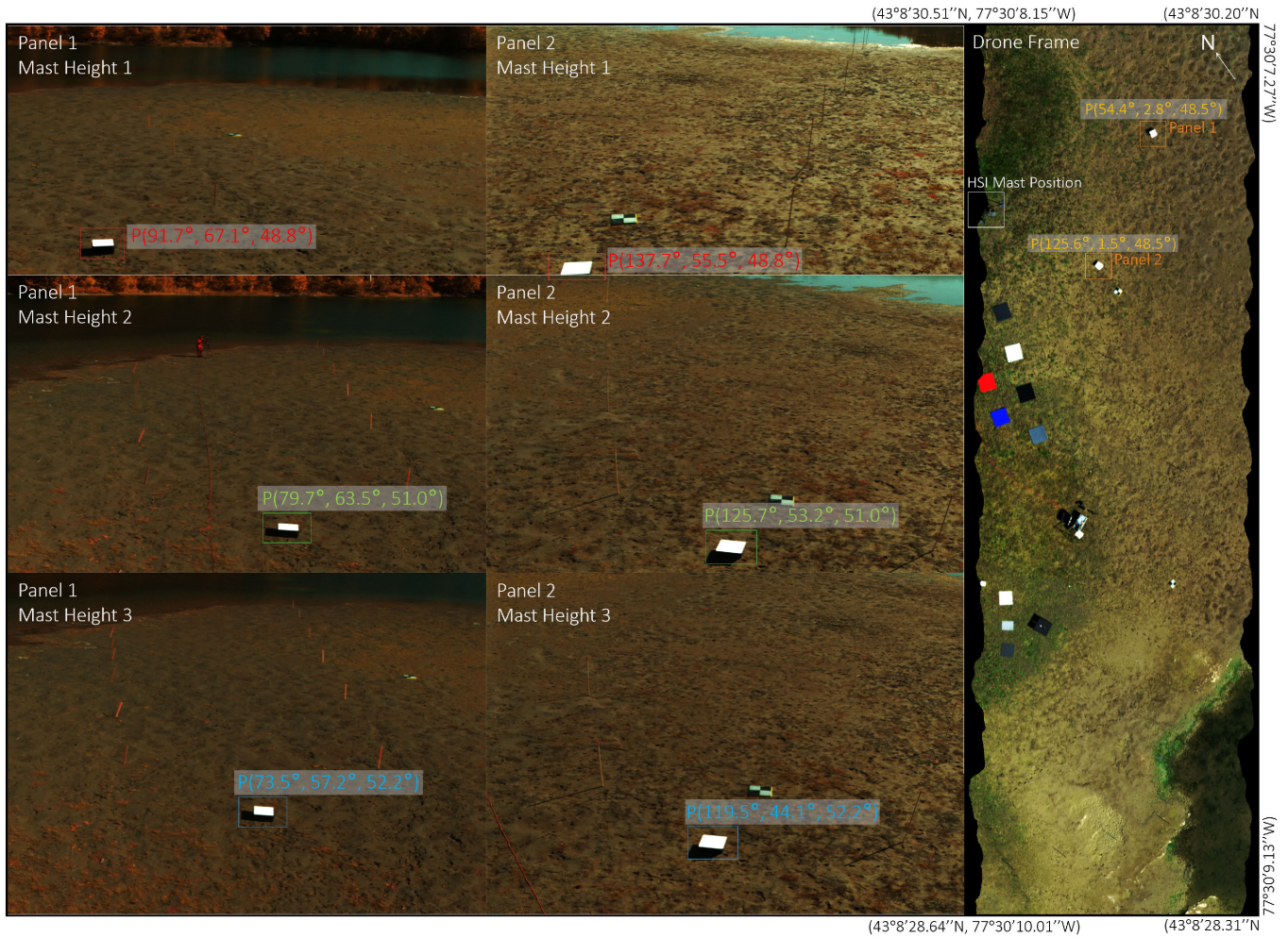
Fig. 7. RGB images derived from the HSI imagery of a mudflat at the RIT Tait Preserve ( 43^{\circ}8'29.53''N , 77^{\circ}30'8.50''W ) during the field experiment using three mast heights from the mast-mounted hyperspectral imaging system [42] and the georectified drone hyperspectral imagery (HSI). The latitude and longitude of the drone frame corners are provided, and panels are identified with their geometries labeled. The colored labels of the panels correspond to the colored spectra in Fig. 8.
