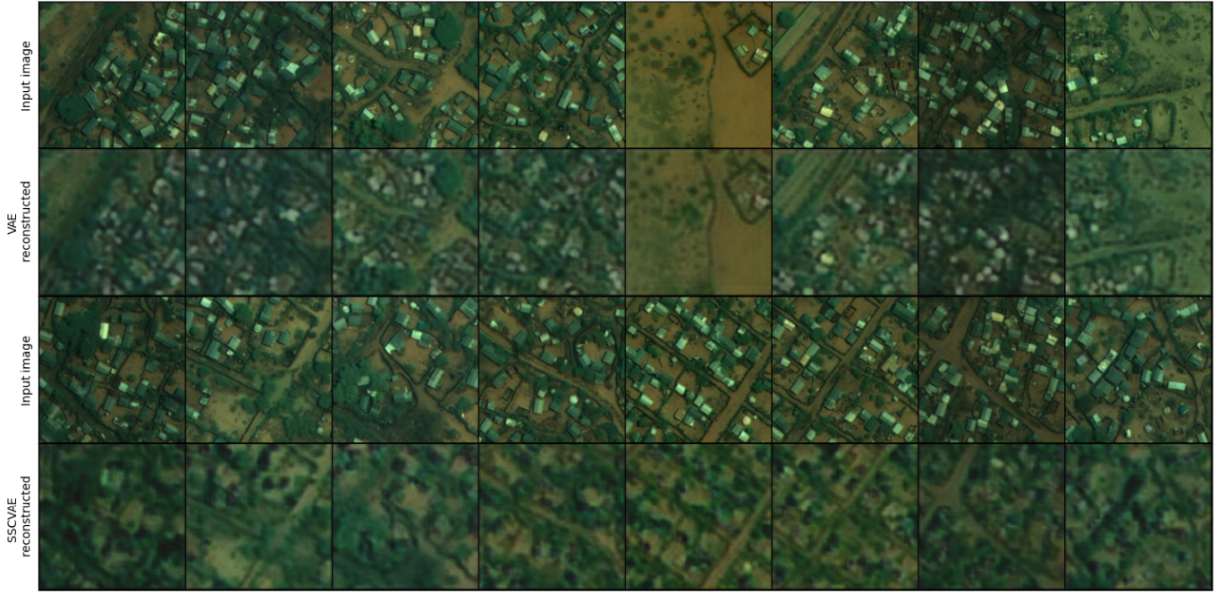
Fig. 3. Image reconstruction with and without self-supervision for randomly selected image chips from the FDP site with complex dwelling structures—Dagahaley. The first image resulted from reconstructions made with classical VAE, while the second image resulted from self-supervised VAE using synthetic anomalies and resultant masks. The first rows are for raw images, while the second rows are for reconstructed images.
