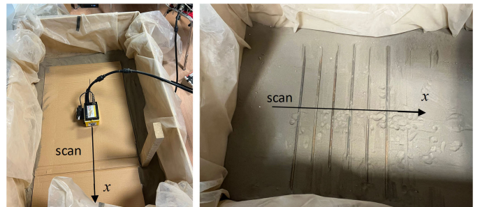
Fig. 12. Photograph of the experimental setup showing the GPR antenna (left panel) and the rebars' arrangement (right panel).
