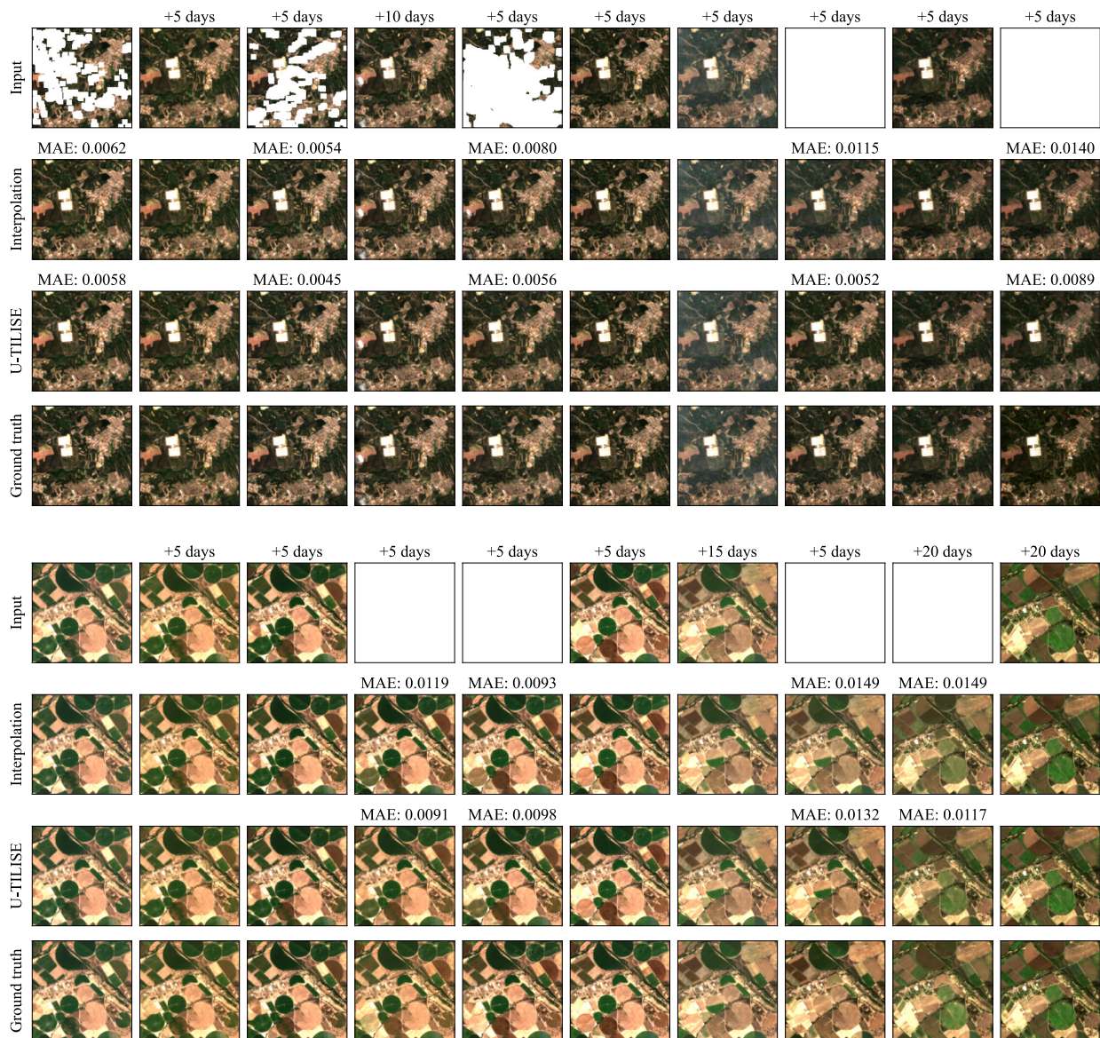
Fig. 3. Visual comparison (true-color RGB composites) of two Sentinel-2 time series of the EarthNet2021 iid test split, gap-filled using either U-TILISE or linear interpolation over time. Rows 1–4 depict a static scene, while rows 5–8 show a scene with sudden land cover changes due to agricultural activities by humans. The number above an image indicates its temporal distance to the previous observation in the sequence or its MAE, evaluated over all pixels that have been masked in the corresponding input image and across all spectral bands (R, G, B, and NIR).
