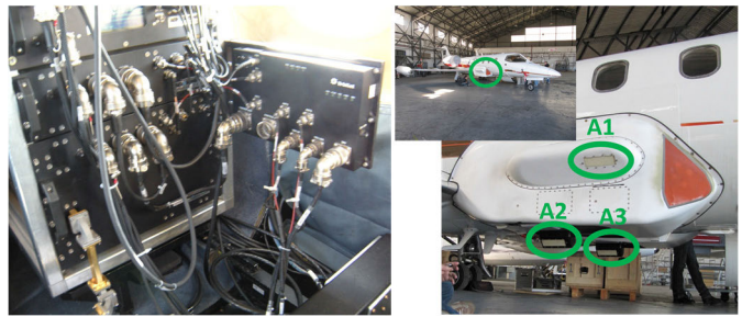
Fig. 7. (Left) InSAeS4 system mounted onboard a Learjet 35A. (Right) Airplane (top) along with a zoom (right) on the three radar antennas, which are highlighted with green ellipses.
