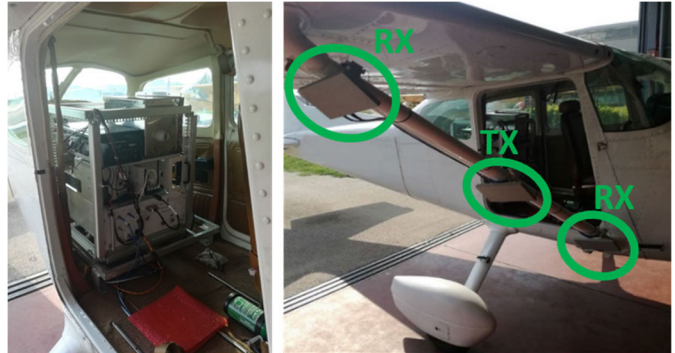
Fig. 8. (Left) AXIS system mounted onboard a Cessna 172. (Right) The three radar antennas, which are highlighted with green ellipses.
