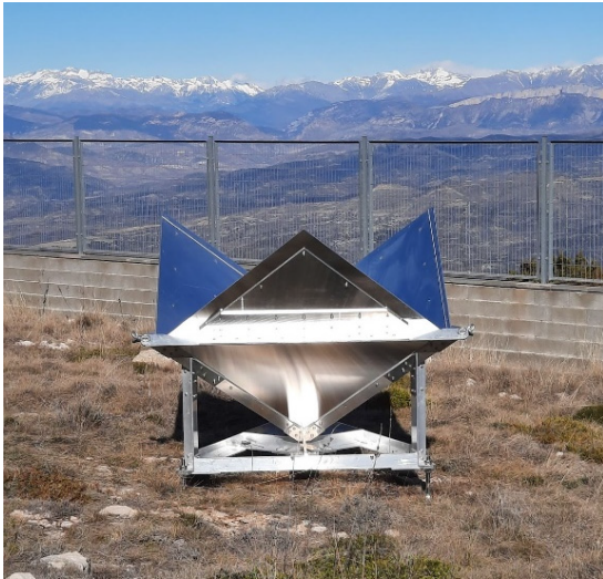
Fig. 2. Picture of the corner reflector at its final location at the Montsec Astronomical Observatory.
