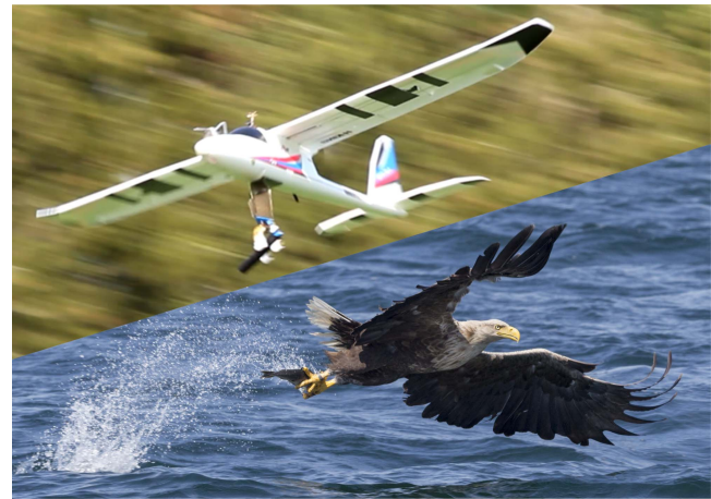
Fig. 1. (Top) UAV with grasped object in the claw and (bottom) eagle having just grasped a fish. Photo of the bird adapted from [7].
