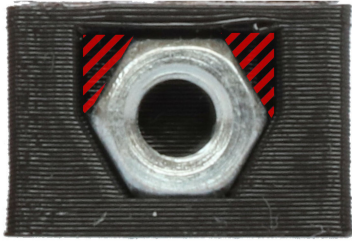
Fig. 3. Cavities generated by our slicing software for horizontal alignment of embedded hexagonal nuts. The volume cross-hatched in red must remain free of plastic during printing to afford vertical insertion of the nut. Note that the volume could be filled after the nut has been placed, but that is not yet supported by our software.
