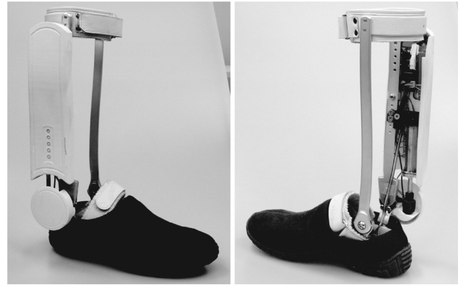
Fig. 3. Overview of SmartAFO. The base frame is an articulated AFO with two metal bars. MRLink is fixed to the lateral bar. A 3-D printed cover is also fixed to the lateral bar, with battery and control circuit embedded inside. A simple mechanism is used to convert the linear force of MRLink into a rotary moment about the ankle joint.
