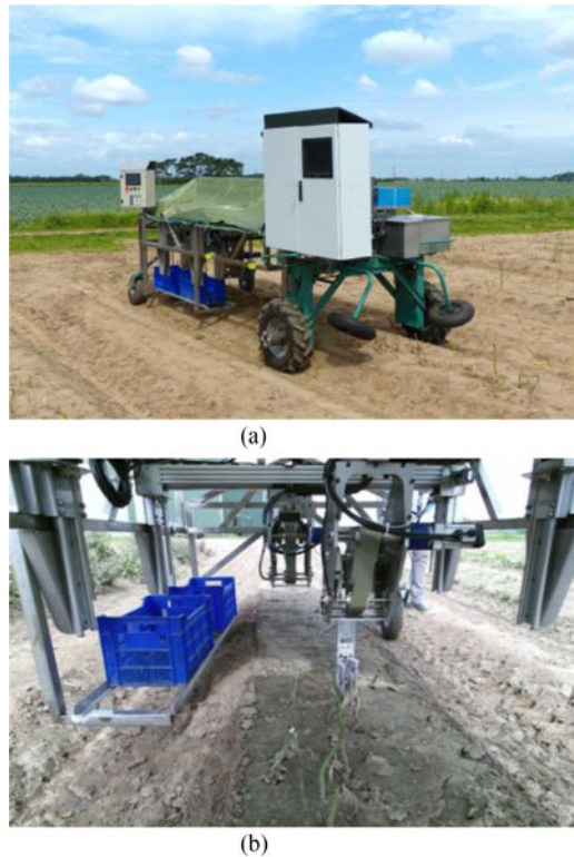
Fig. 9. (a) Robotic harvester driving over an asparagus dam. The asparagus process is seen by the camera. (b) The storage box on the side of the machine.
