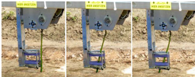
Fig. 10. Illustration of a part of the harvesting process, asparagus stalk approaching and grabbing by one of the harvesting tools.
