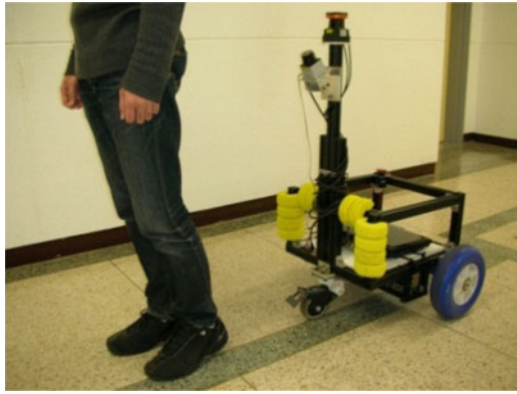
Fig. 12. Marathoner Service Robot equipped with two LRFs for human and obstacle detection.
