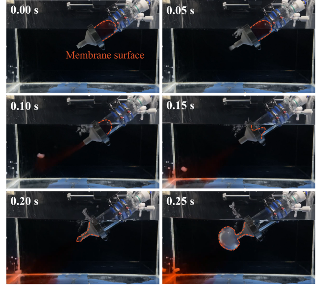
Fig. 13. Water spraying process of the thruster using CM-jet structure is recorded at 0.05 s intervals. The jetted water is precolored with a red dye, to distinguish visually. The outline of the membrane is marked with a dashed line.
