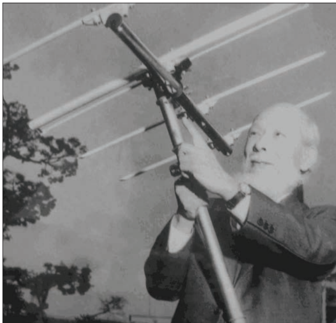
FIGURE 3. Professor Hidetsugu Yagi displays an example of the Yagi-Uda antenna that he and Shintaro Uda invented in 1924–25. (Photo copyright of HYS Engineering Services, Inc., used with permission).
