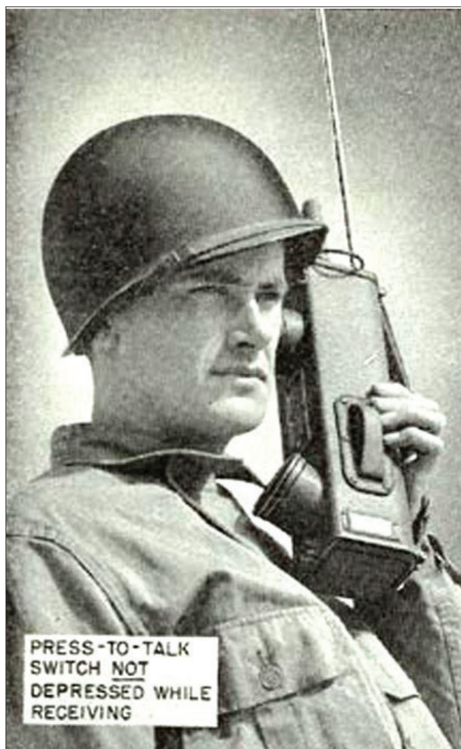
FIGURE 10. Motorola (then called Galvin Manufacturing) created the world's first FM handie-talkies for combat use before WW II. This product was a prelude to the cellphone revolution that amateur radio operators enabled using FM repeaters they deployed across the world throughout the 1960's and 1970's.
