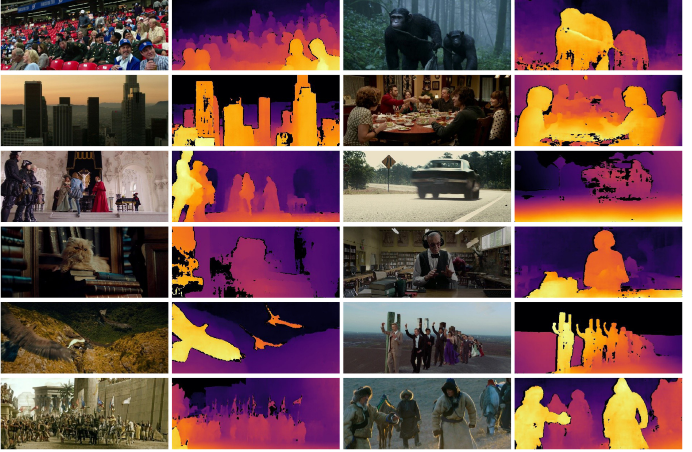
Fig. 2. Sample images from the 3D movies dataset. We show images from some of the films in the training set together with their inverse depth maps. Sky regions and invalid pixels are masked out. Each image is taken from a different film. 3D movies provide a massive source of diverse data.
