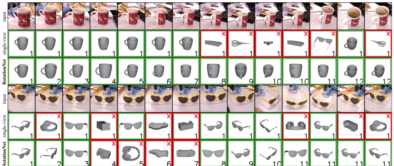
Fig. 16. Exemplar objects recognized using a USB camera. The second and fifth rows show 3D models in the estimated category and pose from a single view, whereas the third and sixth rows show those estimated using multiple views. The number in each image indicates the number of views used for predictions. Failure cases are shown in red boxes.
