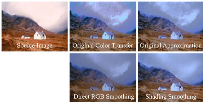
Fig. 9. Color transfer enhancement. A source image is color transferred by [63] with some noticeable imperfections (on the clouds). This issue is fixed by approximating the original color transfer effect with a shading-smoothed shading homography. Visually, the enhanced result also preserves more texture details compared with the result obtained by directly smoothing the original approximation RGB.
