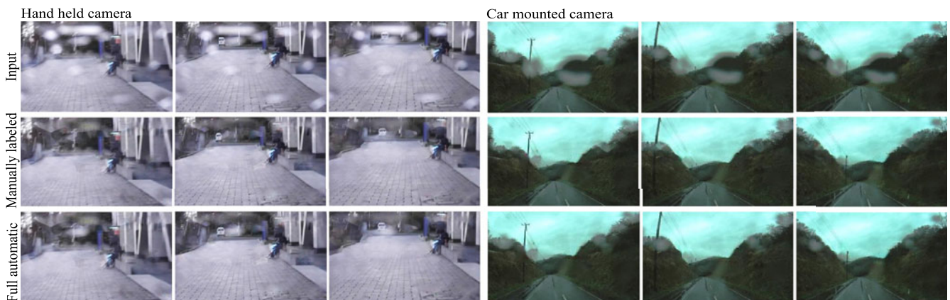
Fig. 23. The raindrop removal using our method. First row: the input sequence. Second row: the removal result with the raindrops manually labeled. Third row: the removal result with the raindrops automatically detected.
