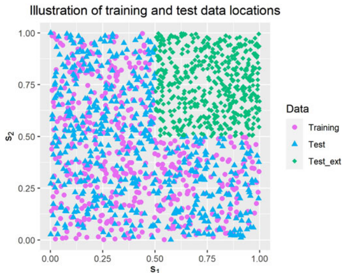
Fig. 1. Example of locations for training and test data for the spatial data. ‘Test’ and ‘Test_ext’ refers to locations of the interpolation and extrapolation test data sets, respectively.
