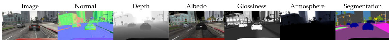
Fig. 5. For a rendered image (left), G-buffers represent information on geometry (e.g., normal, depth), materials (e.g., albedo, glossiness), and lighting (e.g., atmosphere). A semantic segmentation, which can be derived from the G-buffers [27], [87], provides further high-level information on the scene.
