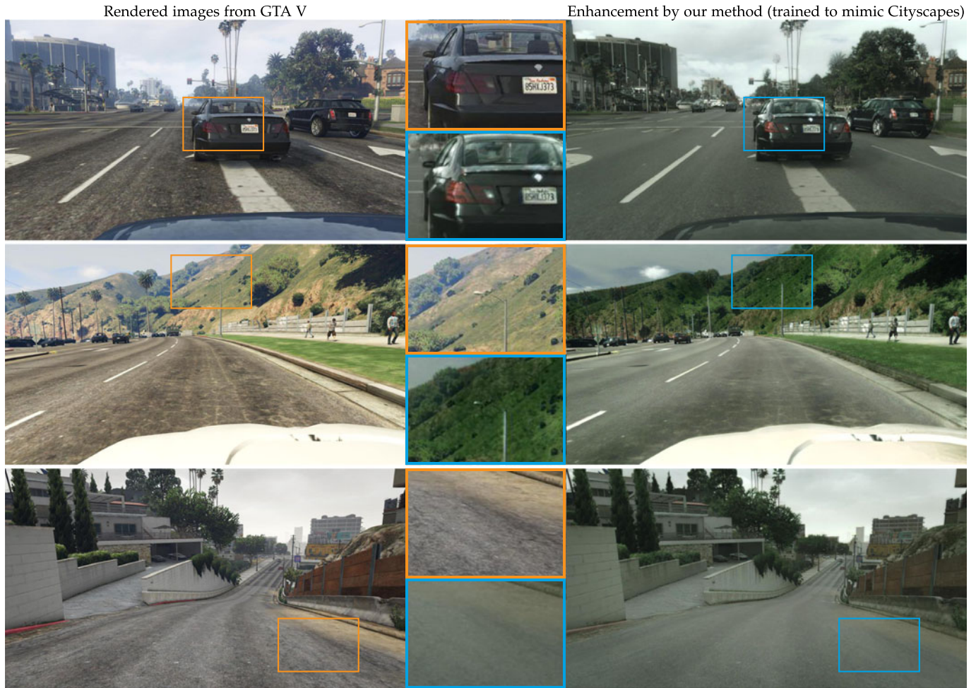
Fig. 1. We train convolutional networks to enhance the photorealism of rendered images, using intermediate buffers produced by a conventional rendering engine. Left: frames from a modern computer game (GTA V) [27]. Right: same frames enhanced by our approach to mimic the style of Cityscapes [28]. Enhancements by our method are semantically consistent and non-trivial. For example, our method adds gloss to cars (1st row), reforests parched hills to mimic German climate (2nd row), and paves roads with smoother asphalt (3rd row). Insets magnify marked regions.
