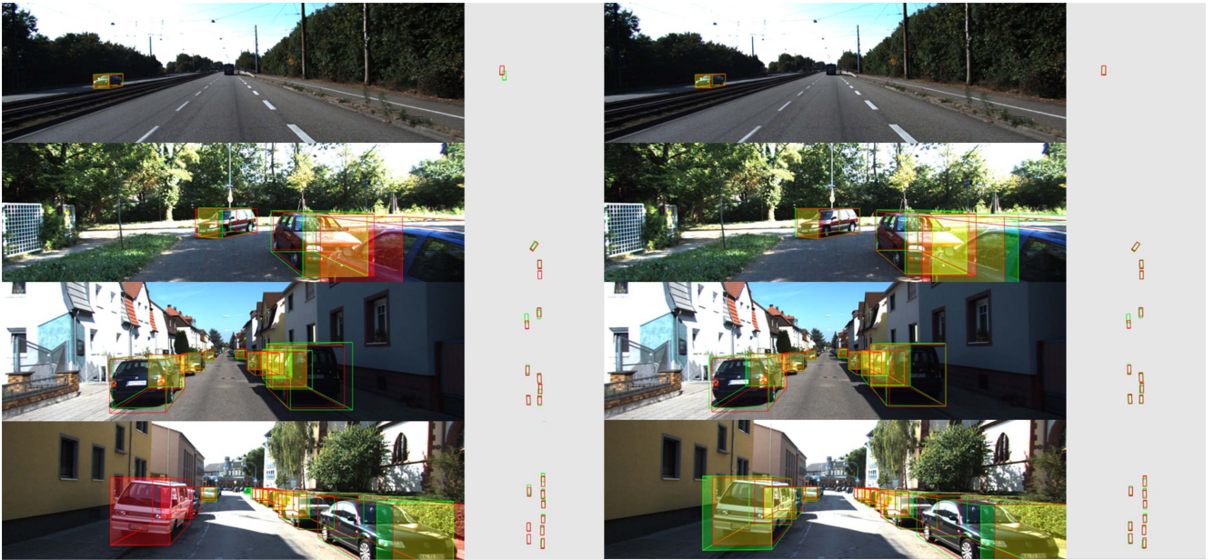
Fig. 6. The proposed method (right) and the baseline (left) are compared in terms of their predictions on both the image view and BEV, as shown in the qualitative results. The predicted boxes are represented by green, while the ground truth boxes are in red.
