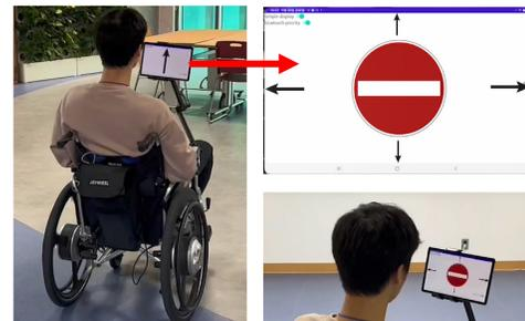
Fig. 2. Left: gaze direction control electric wheelchair for the disabled. Gaze estimation is based on an appearance-based method. Right: control screen of the wheelchair. The user determines the direction and movement of the powered wheelchair by staring at the arrow. Courtesy of Jaehyun Kim.
