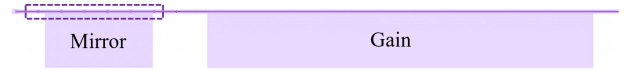
Fig. 9. A schematic view of the Single-mirror SFP device with slotted perturbations highlighted.
