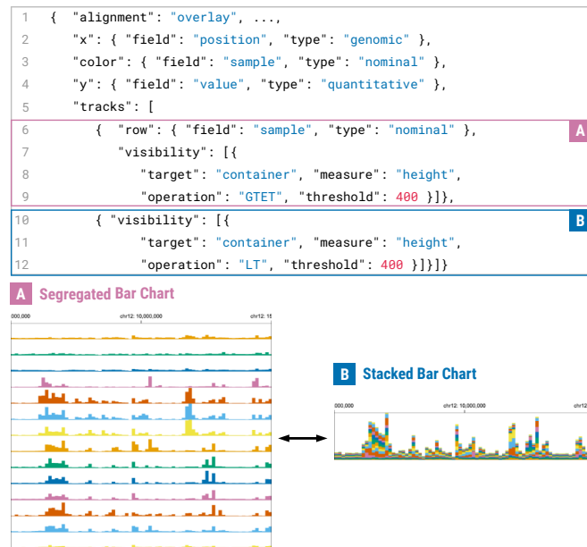
Fig. 9. An example of track-level responsive designs with a spec (top) and a corresponding visualization (bottom). A segregated bar chart switches to a compact visualization, i.e., stacked bar chart, in a smaller screen, focusing on showing the hotspots on the genomic axis.
