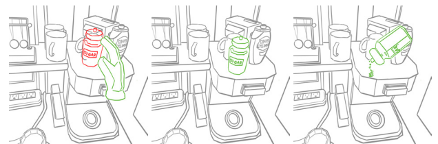
Fig. 6. Tomato Presence in action. As the user touches the sugar shaker (left), it changes colour. As they grab it (middle), their hand disappears. They can then manipulate the object (right). The hand re-appears when the object is released.
