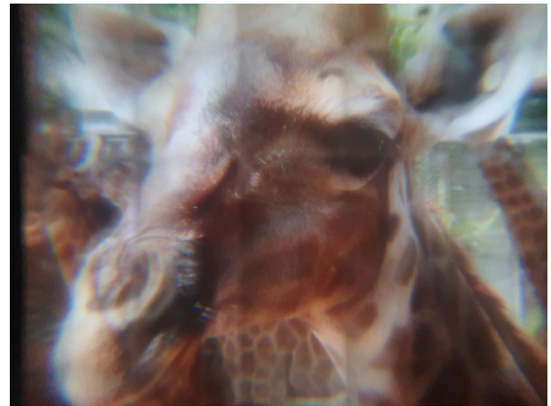
Fig. 15. The display result of VR glasses prototype. The camera is located at the center of the eye-box. The photo is a screenshot of a video, which is provided in supplementary media.
