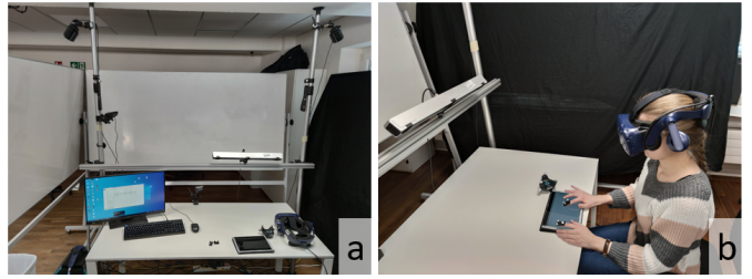
Fig. 5. The study setup. a: setup with motion tracked tablet, fiducials for the fingers and HTC Vive Pro Eye to the right. The lighthouse systems were placed on the ceiling around the table and the Optitrack system on a bar above the table. The monitor, keyboard and mouse to the left were operated by the experimenter to start individual conditions. b: Participant during the study.
