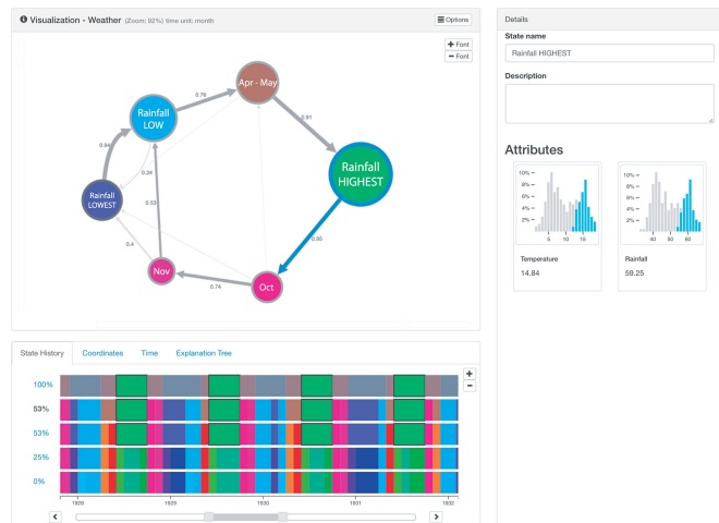
Fig. 3. The visualization consists of 3 panels. The central panel visualizes the data through a Markov chain at the current scale. The bottom panel shows a cross-scale historical overview of the dataset using an icicle plot . States on the two panels are associated by color. The right panel visualizes properties of the currently selected state (blue border).
