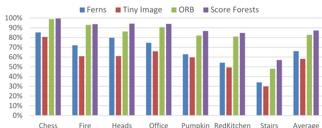
Fig. 7. Comparison with offline LbAs: Compared to our real-time fern-based method, the two offline landmark-based approaches perform favorably. Though, their applicability is limited to scenarios of revisiting a previously reconstructed scene after training.
