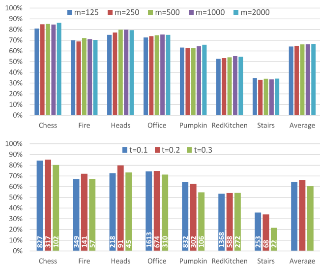
Fig. 8. Effect of number of ferns and harvesting threshold: Relocalization performance when varying the number of ferns m (top graph) and changing the keyframe acceptance threshold t (bottom graph). Initially increasing the number of ferns improves performance, which levels off after m=500 . The threshold t influences the number (in white), and thus, the density of keyframes. Optimal coverage seems to be obtained with t=0.2 (see also Fig. 2 for a visual example).
